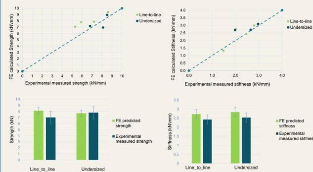
Figure 9 Scatter plots and bar charts of strength and stiffness for FE results against experimental data
