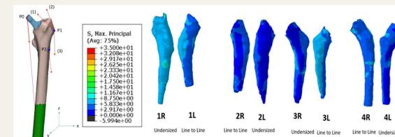
Figure 11 Stress distribution under physiological loading conditions
