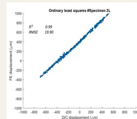
Figure 10 Regression analysis on the displacement data using DIC and FE results
